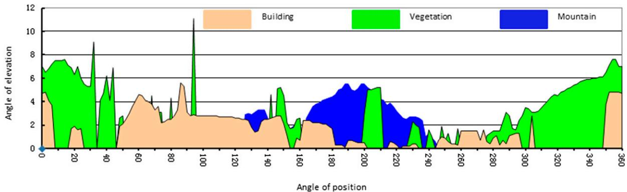
FIG. 9. Angles of elevation of obstacles surrounding Donggang station, Jilin Province.
