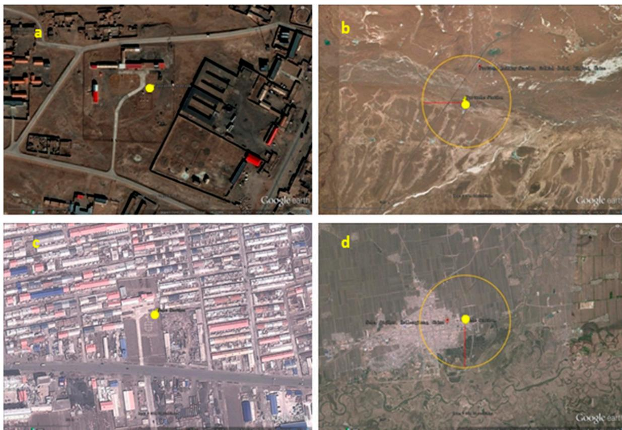
FIG. 7. Distributions of built-up areas inside the 2-km-radius circular scope at (a),(b) Tuotuohe station, Qinghai Province, and (c),(d) Nehe station, Heilongjiang Province, as seen in the Google Earth pictures. The scales are approximately 1:100 m for (a) and (c) and 1:3000 m for (b) and (d). Yellow points indicate locations of the observational stations, and red lines in (b) and (d) denote the 2-km radius from the observational stations located at the centers of the yellow circles.
